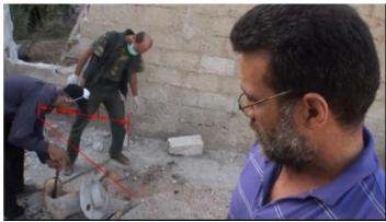
This results in an angle from the wall equal to: Arctan  $(1.8/3) = 31^{\circ}$ . Since the wall has an azimuth of 82° (or 262°), the trajectory azimuth is around 293°.
