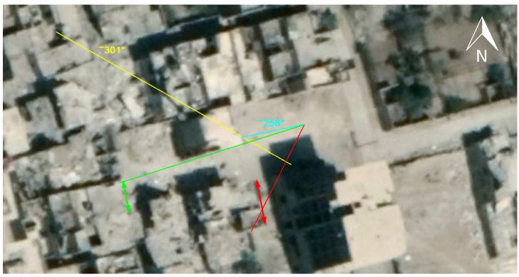
When matching these features to the satellite image, the azimuth of the crater can be estimated at 121° (or 301° when measured in the opposite direction). We estimate an error of 5° in each direction, due to errors in the camera angle, projection, or crater shape.
