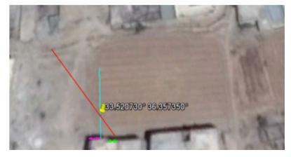
The crater points (red line) approximately to the far part of the next section of the building (green). In this way the azimuth can be roughly estimated at 137°.
