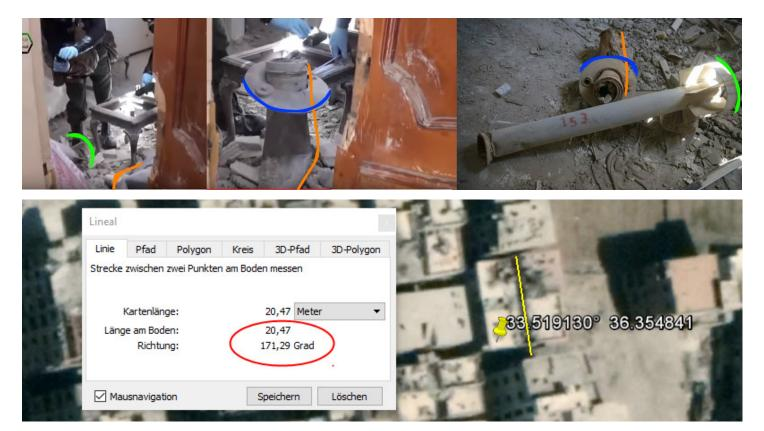
The penetrated western wall has an azimuth of about 171°. To be able to penetrate this wall without going through the northern wall, and continuing to the floor below, the trajectory azimuth can not exceed 154°. Since the western wall impact may have diverted the rocket from its flight path, smaller azimuths are also considered possible.
