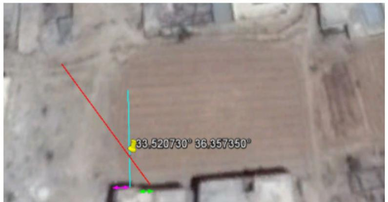
The crater points (red line) approximately to the far part of the next section of the building (green). In this way the azimuth can be roughly estimated at 137°.
