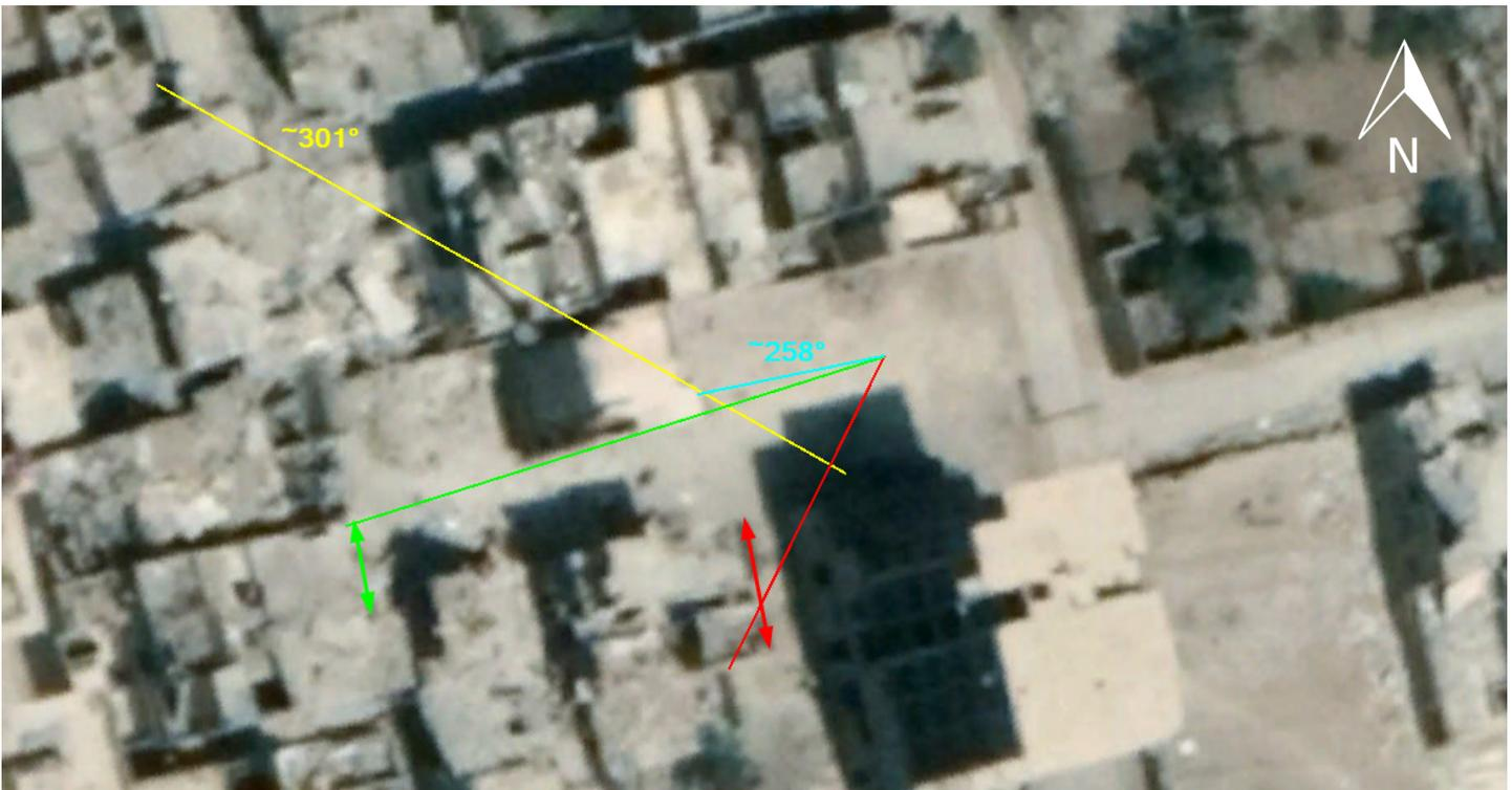
When matching these features to the satellite image, the azimuth of the crater can be estimated at  $121^\circ$  (or  $301^\circ$  when measured in the opposite direction). We estimate an error of  $5^\circ$  in each direction, due to errors in the camera angle, projection, or crater shape.
