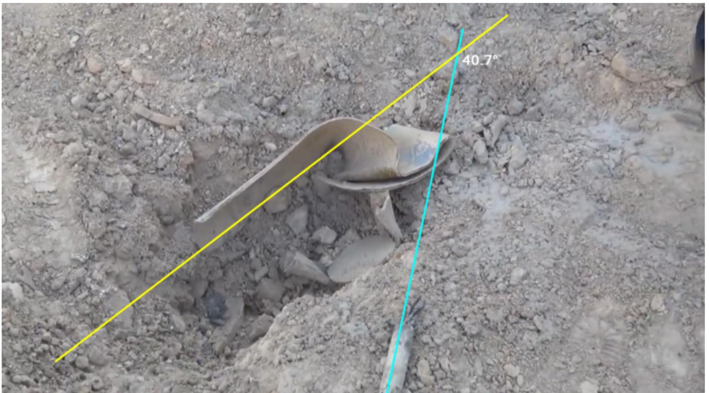
A re-creation of the crater as a 3D model using Autodesk point-cloud technology reveals the angle between the two pieces to be 42°.
